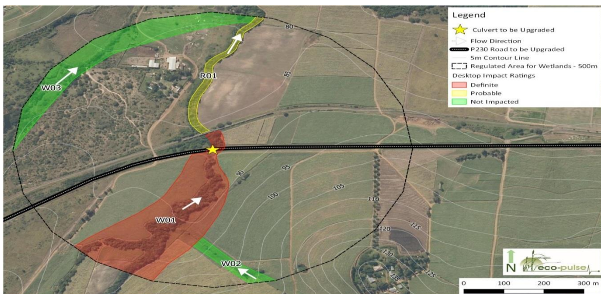
Figure 7-1: Impact screening and rating of desktop mapped watercourses within the 500 m regulated area for wetlands in terms of Section 21 c and/or i water use (National Water Act) for the culvert
